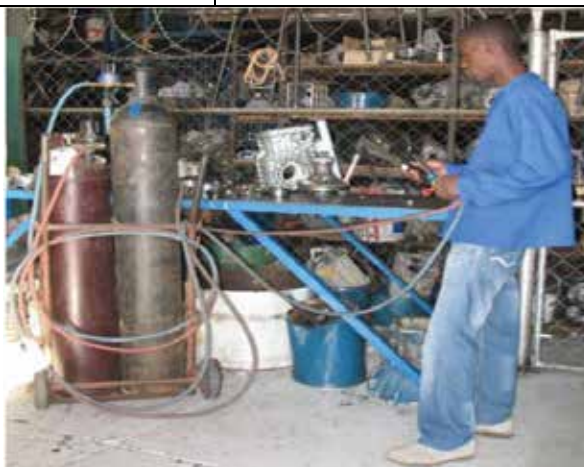
Easy: slicing through steel with an oxy-acetylene flame.
